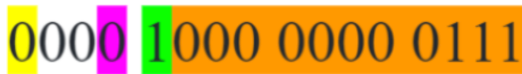
Figure 30: An image of a possible packet header. In this image, the orange bits represent the length, the green represents the CRC, the purple represents whitening, and the yellow represents whether or not the packet includes a payload or not.
