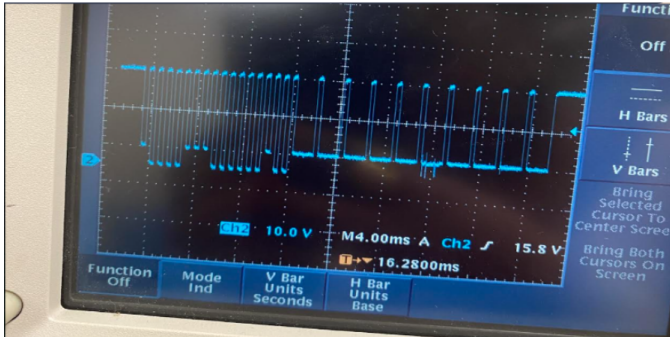
Fig. 13. This image depicts captures taken from the oscilloscope when the pull station was in an idle state.
